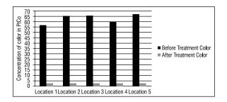
Figure 1: Color of municipal wastewater before and after treatment
