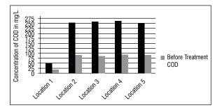
Figure 4: COD of municipal wastewater before and after treatment
